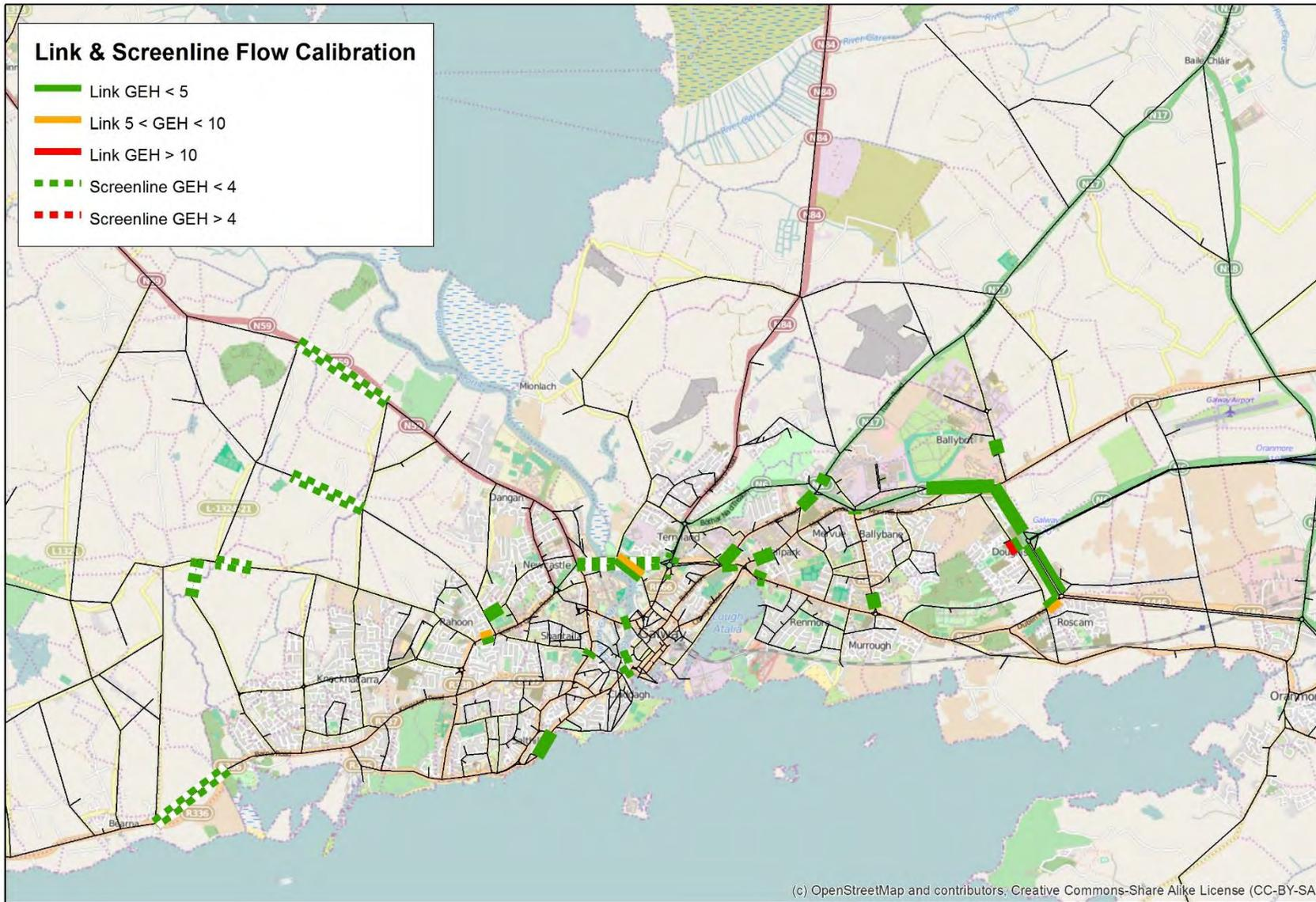
Figure 4.4.2: Link Flow Calibration – Morning Peak Hour (zoom)
