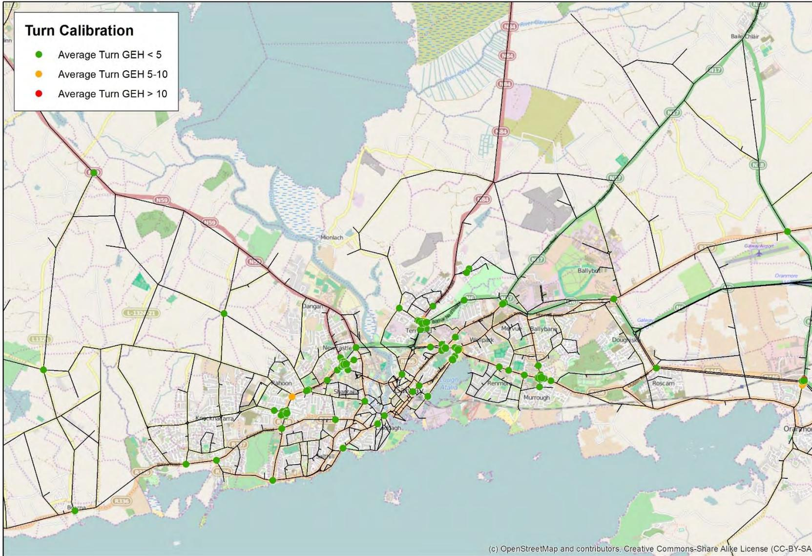
Figure 4.4.6: Turn Flow Calibration – Morning Peak Hour (zoom)
