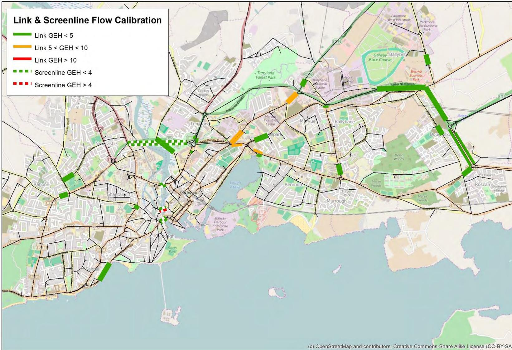
Figure 4.4.5: Turn Flow Calibration – Morning Peak Hour (wide)
